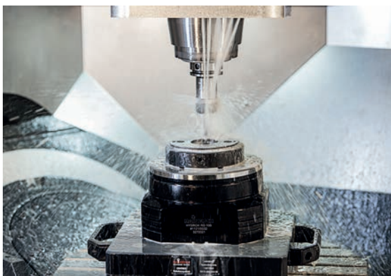
HYDROK hydraulic stationary chuck in use
