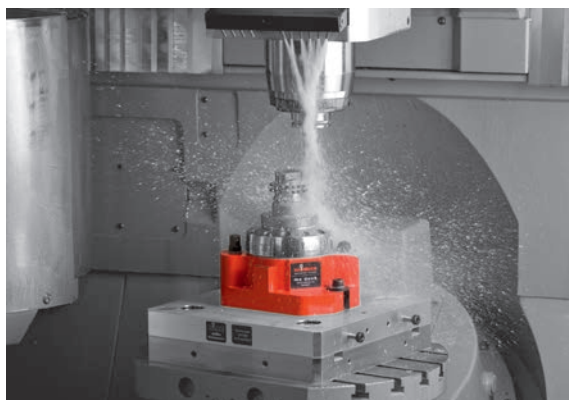
ms dock mandrel actuating unit in use
