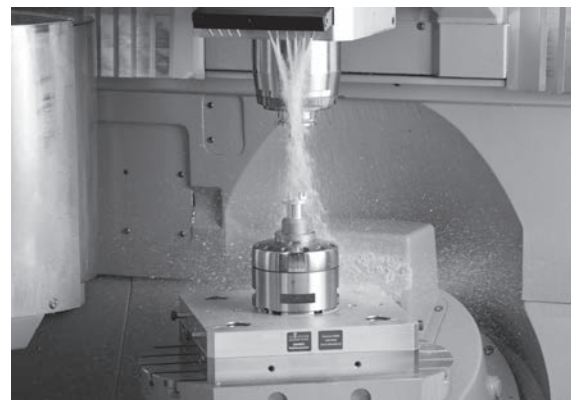
hs dock mandrel actuating unit in use
