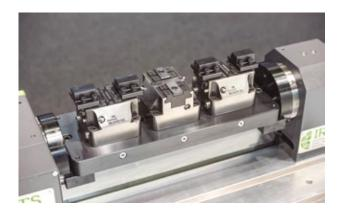
Another common application is in vertical machining centers to which we can add a fourth axis. Normally, by using a rotary table and a plate with some BLOCK-SCs in both faces, saving machine downtime.
