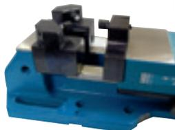
Possibility of working with machined soft jaws according to the shape of the work piece.
