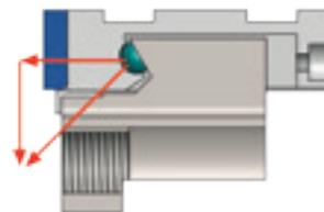
The ARNOLD MAT has a descending clamp system to avoid that the clamped part lifts up. This is a semi-sphere installed between the moveable jaw and the spindle shoe. When the clamping force is carried out by the spindle, this pressure is divided in two directions, one of which pulls down on the work-piece.
