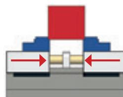
The spindle within the base jaws, just at the top of guide support, allows for applied force to be as close as possible to the piece to be machined. This means that the torque power is used to its fullest.
