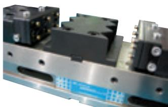
Possibility of working with machined soft jaws according to the shape of the workpiece.
